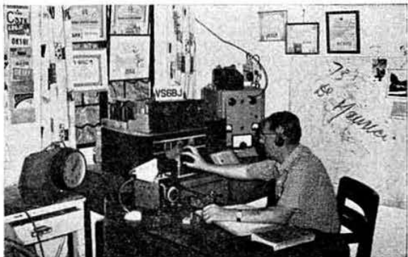
The equipment at VS6BJ comprises an R.C.A. AR88 receiver, BC221 frequency meter and a Labgear LG300 transmitter.
