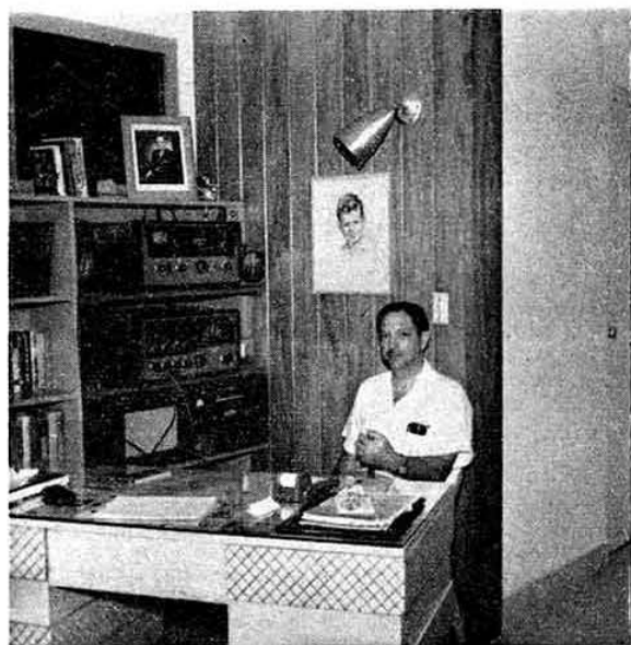
HP1GP in the Republic of Panama uses a Hallicrafter transmitter, Collins 75A4 receiver and Telrex four-element beams for 14, 21 and 28 Mc/s. Operation is principally on s.s.b.
